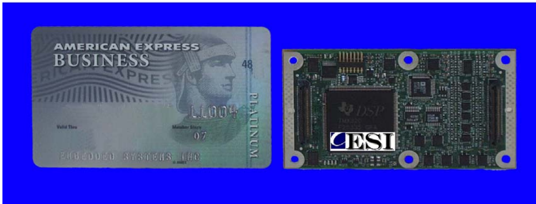
Figure 1 - Dual-Axis Servo Controller – sub Credit Card Sized
